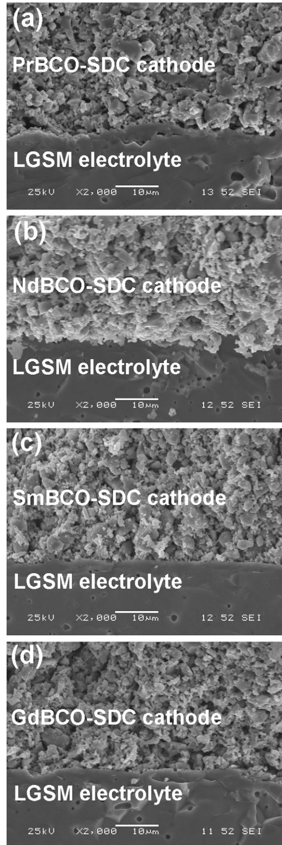
Fig. 10. SEM micrographs of the cross-sections of the cathode/electrolyte interface after the cell testing at 700 °C for 20 h: (a) PrBCO-SDC/LSGM; (b) NdBCO-SDC/LSGM; (c) SmBCO-SDC/LSGM; and (d) GdBCO-SDC/LSGM.
